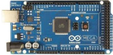
Gambar 3. Arduino Mega 2560[5]
