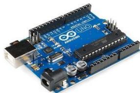
Gambar 1. Modul Kit Arduino UNO
