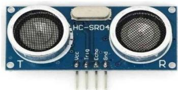
Gambar 5. Sensor Ultrasonik HC-SR04
