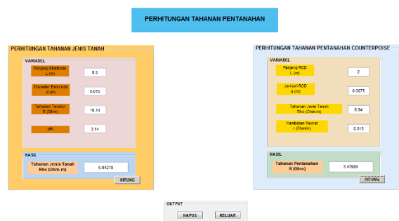
Gambar 8. Perhitungan Tahanan Pentanahan Tower 39
