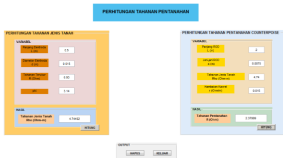
Gambar 7. Perhitungan Tahanan Pentanahan Tower 70
