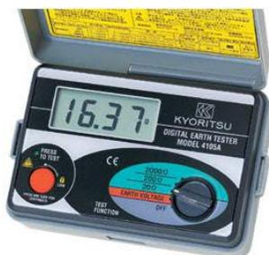
Gambar 8. Alat Ukur Pentanahan (*Earth Tester*)
