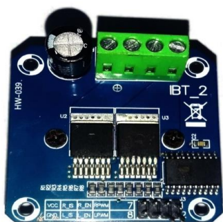
Gambar 2. Motor Driver BTS7960
