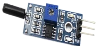
Gambar 6. Sensor Getar SW-11810P (Sumber: Najmurrohman, 2018)
