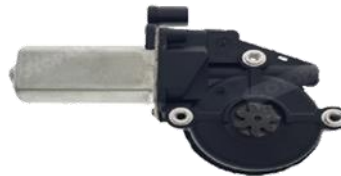
Gambar 7. Motor DC Power Window (Sumber: https://kumparan.com/kumparanoto/bentuk-fisik-motor-power-window-mobil/ )
