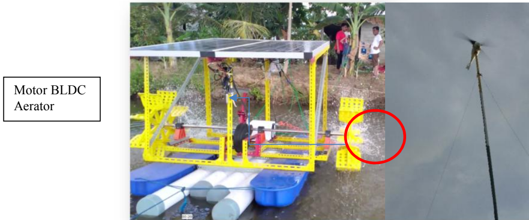
Gambar 1. Motor BLDC Aerator Sistem Hybrid Photovoltaic-Wind Turbine
