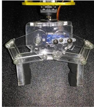
Gambar 7. *Gripper* Prototipe Robot Manipulator
