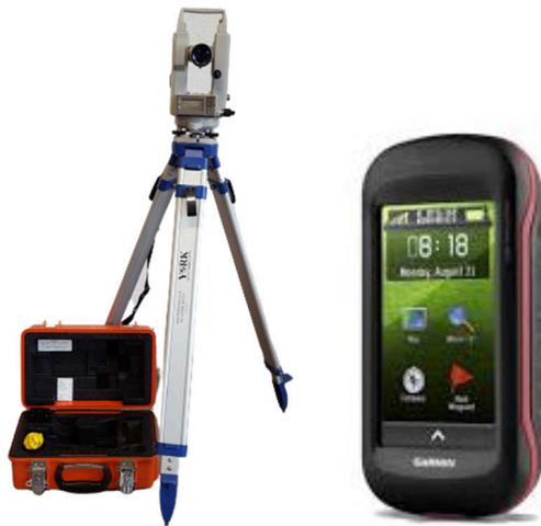
Gambar 1. Alat digital theodolit Sokkia DT-6 dan GPS Garmin Montana 680
