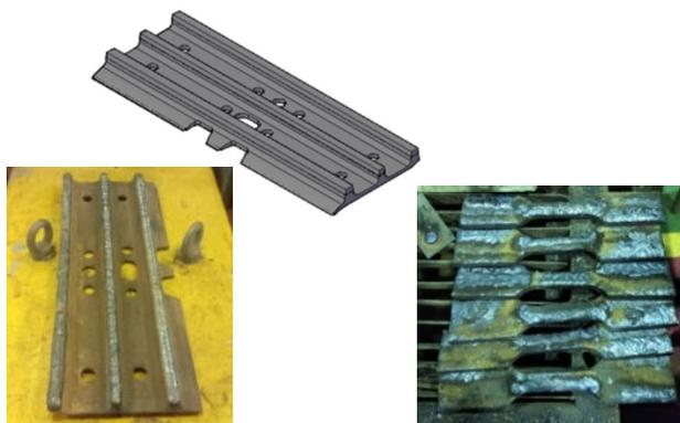
Gambar 2. Desain, hardfacing, dan specimen tensile
