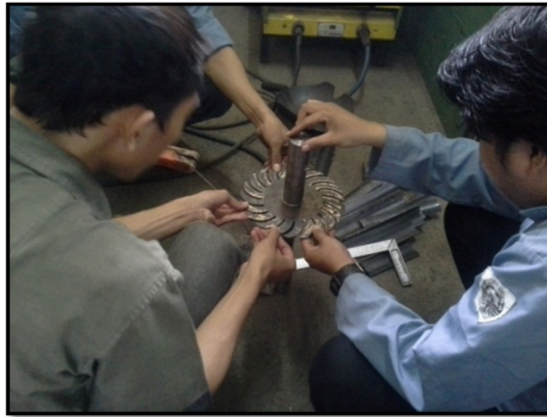
Gambar 2. Proses Perakitan Runner turbin.
