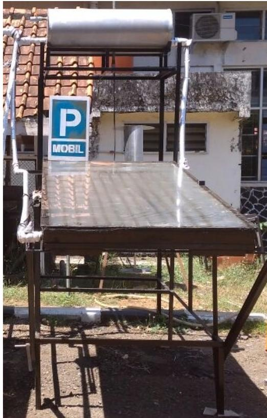
Gambar 2. Alat uji sistem *solar water heater*
