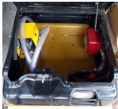
Gambar 4. Refill Fuel Elektrik Unit Excavator 313D
