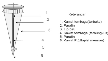
Gambar 1. Desain Elektroda Tipe Kawat Terlapis
