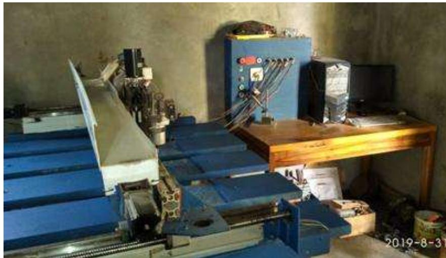
Gambar 3. Mesin milling CNC
