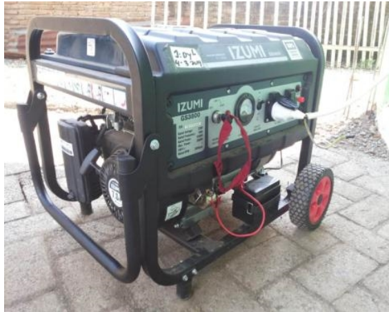
Gambar 1. Generator Set 2800 Watt
