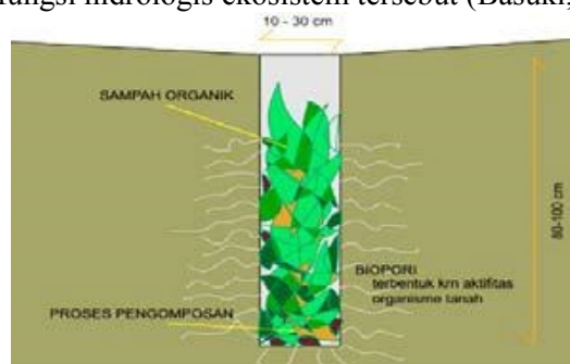
Gambar 1. Sketsa Penampang Lubang Resapan Biopori
