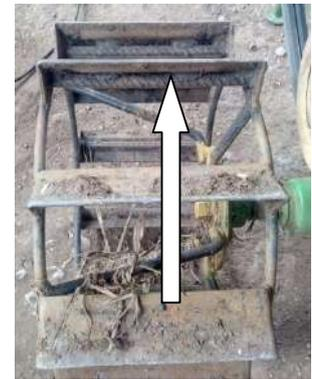
*Sirip roda sering bengkok & retak*
