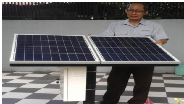
Gambar.6 Modul Solar Cell 2 x 50 Wp
