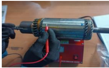
Gambar 10. Pengujian Ground Armature
