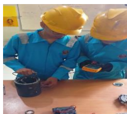
Gambar 8. Field Winding Ground Test
