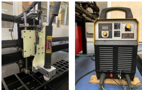
Gambar 1. Head Torch Plasma dan Inverter cut-100 A
