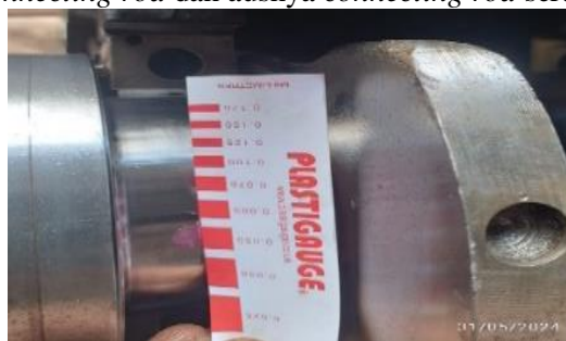
Gambar 2. Hasil pengukuran Clearance oil connecting Rod = 0.50 mm (standart 0.63 – 0.75 mm)
