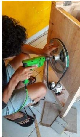
Gambar 2. Pemasangan belt Box Dryer
