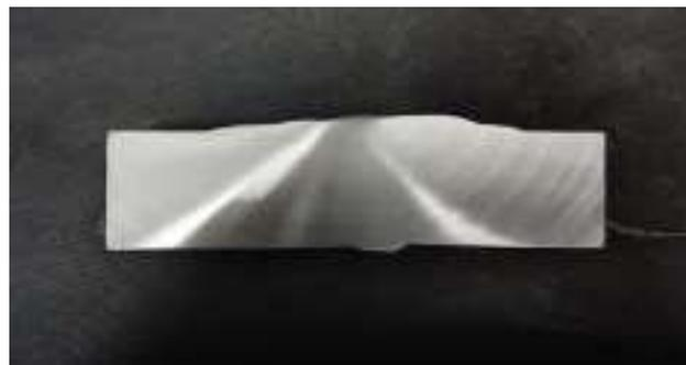
Gambar 8: Spesimen Macro Examination
