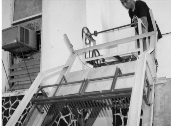
Gambar 1. Sistem Trash Rake Semi Otomatis
