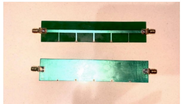
Figure 6. Fabricated fifth-order optimum distributed HPF prototype.
