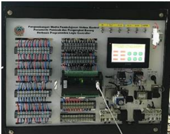
Figure 9. PLC and HMI circuit
