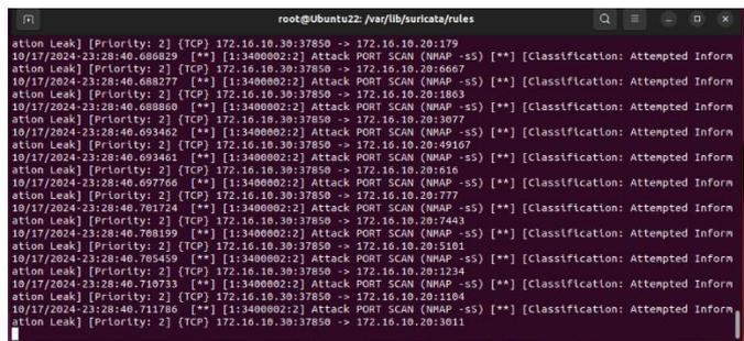
Figure 5. Alert Port Scanning Attack
