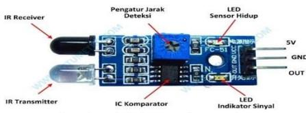
Gambar 2.3 Sensor Infrared
