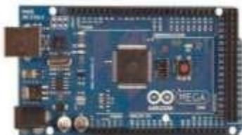
Gambar 1 Arduino Mega 2560
