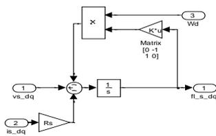
Gambar 5. Model fluks stator motor
