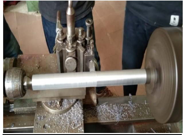
Figure 4. The Workpiece Is Being Turned
