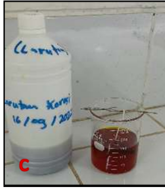
FIGURE 2 Immersion of specimens in \text{FeCl}_3 solution.
