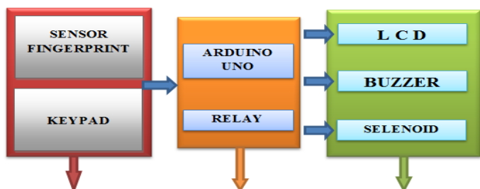
Figure 4: Block diagram of the circuit
