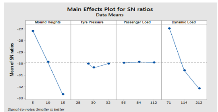
Figure 8. Main Effects Plot of S/N Ratio on Vibration Acceleration RMS Suspension value
