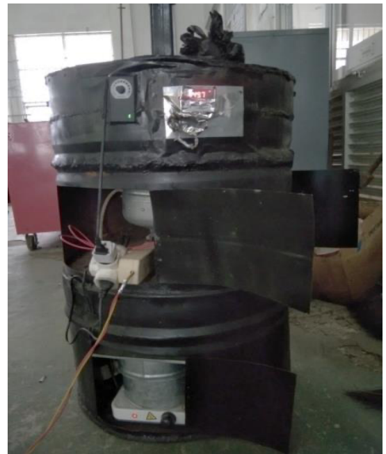
Figure 3. The myristica fragrans seed dryer uses an electric stove
