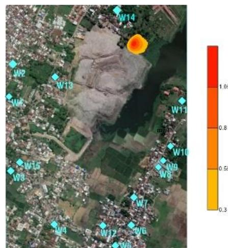
Figure 17. The pumping result at layer six with a flow rate of 1500 m<sup>3</sup>/day for 15 months.
