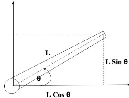
Figure 2. Kinematic 1-DOF
