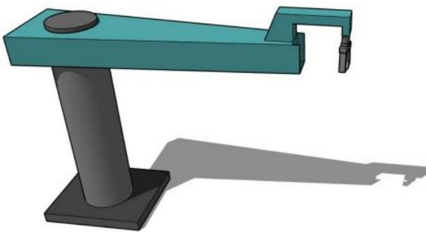
Figure 1. Design of Robot Manipulator 1-DOF
