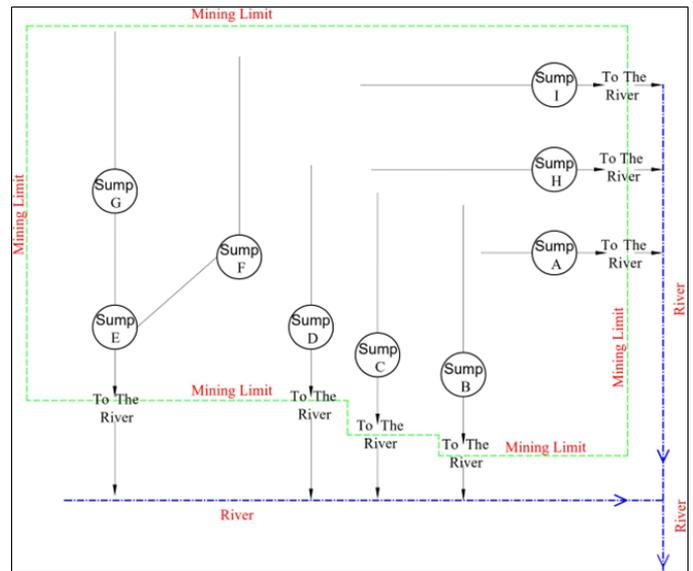
Figure 4. Sump Flow Direction Scheme (Sediment Trap)
