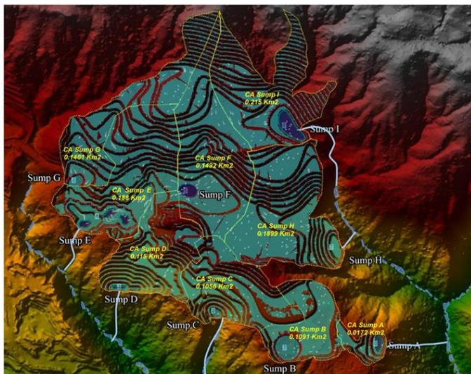
Figure 3. Layout Plan and Catchment Area of Sump.
