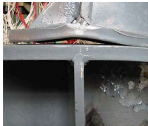
Figure 5. Prying action Source: Adapted from [26]
