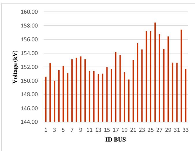
Figure 1. Graph of Voltage on the 150 kV Bus System at Maros and Sidrap Load Release
