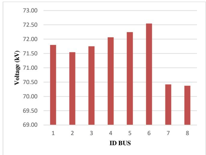
Figure 2. Graph of Voltage on the 70 kV Bus in the Sulsebarar system at the time of releasing Maros and Sidrap loads
