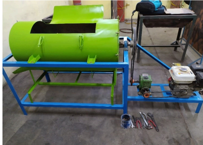
Figure 2. Manufacturing result of grain dryer machine
